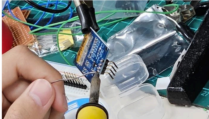
Figure 2: Soldering the LED
